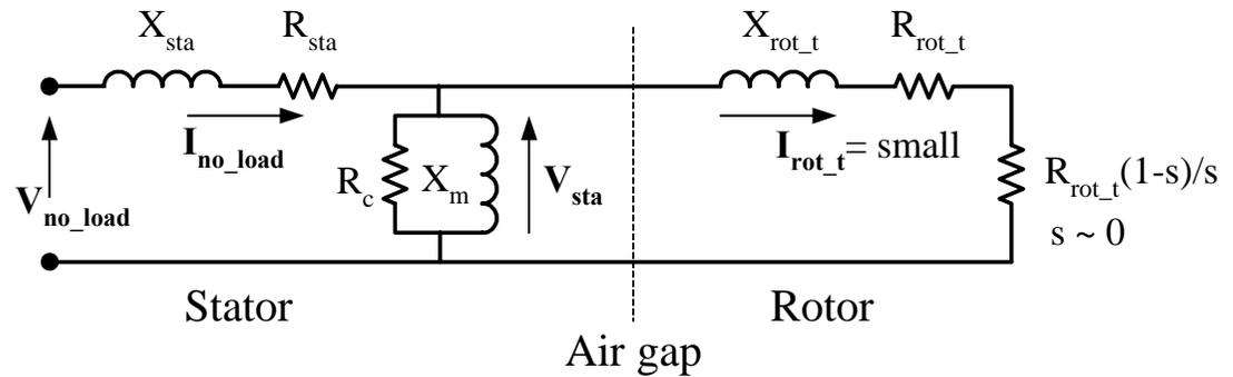
**Fig. 30 Simplified equivalent motor circuit in no-load test**
