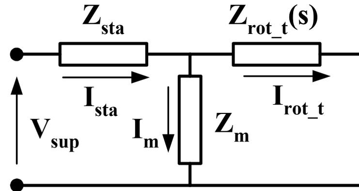
**Figure 7.22 Simplified motor equivalent circuit.**
