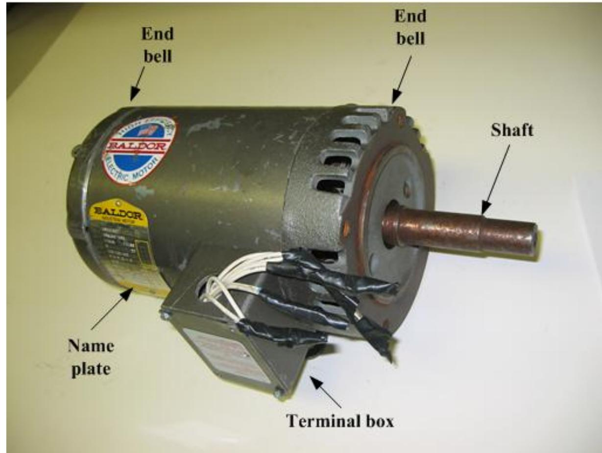
Figure 1 Single-phase induction motor.
