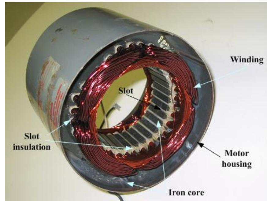
**Figure 6** Single-phase stator with main windings.
