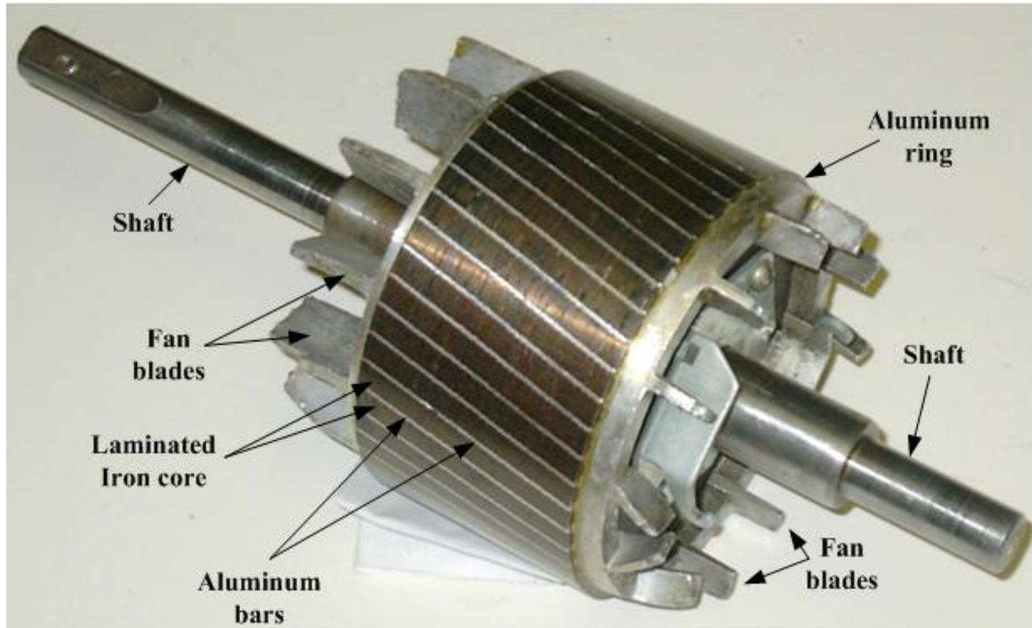
**Figure 10 Squirrel cage rotor.**
