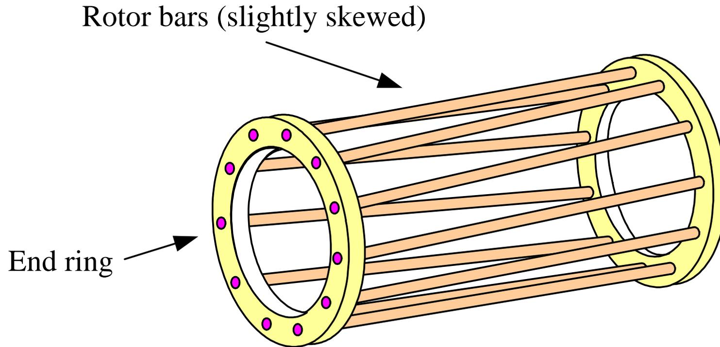
**Figure 9 Squirrel cage rotor concept.**
