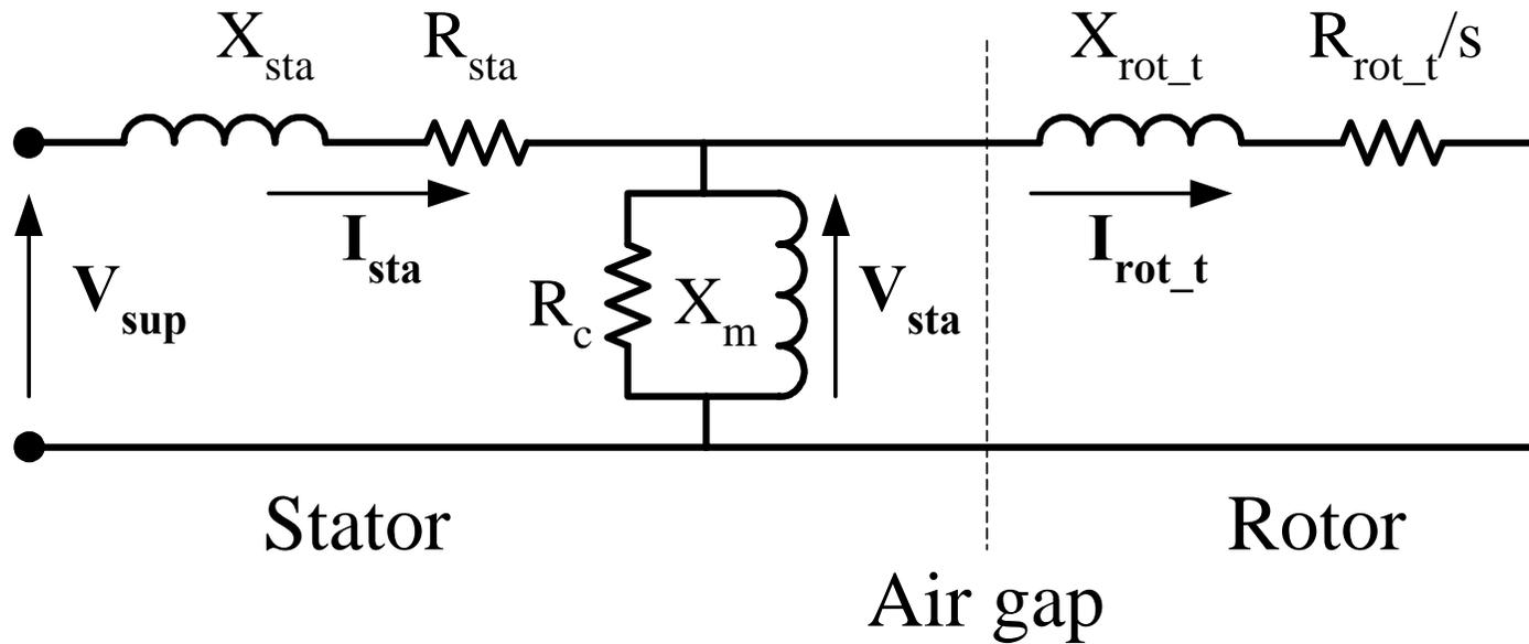
**Figure 19 Simplified equivalent circuit of a three-phase induction motor.**
