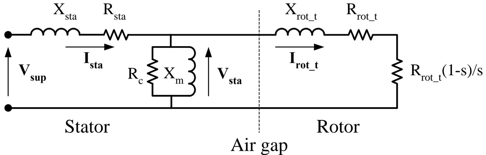
**Figure 20 Final single-phase equivalent circuit of a three-phase induction motor.**
