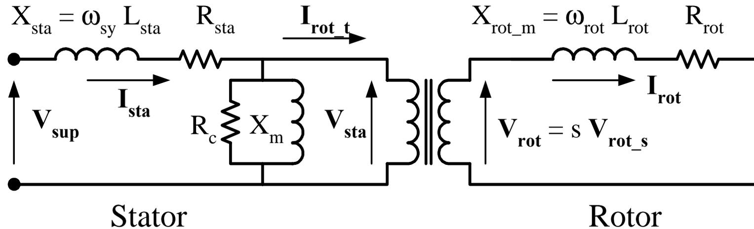
**Figure 17 Single-phase equivalent circuit of a three-phase induction motor.**
