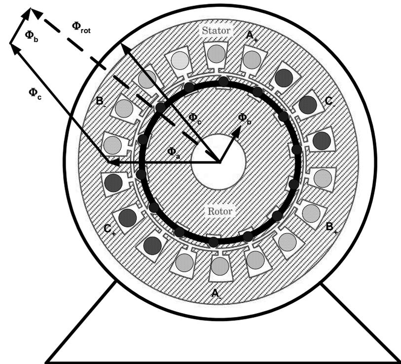
**Figure 12 Three-phase winding-generated rotating magnetic field.**
