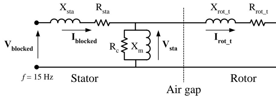
Figure 32 Simplified equivalent motor circuit for blocked-rotor test
