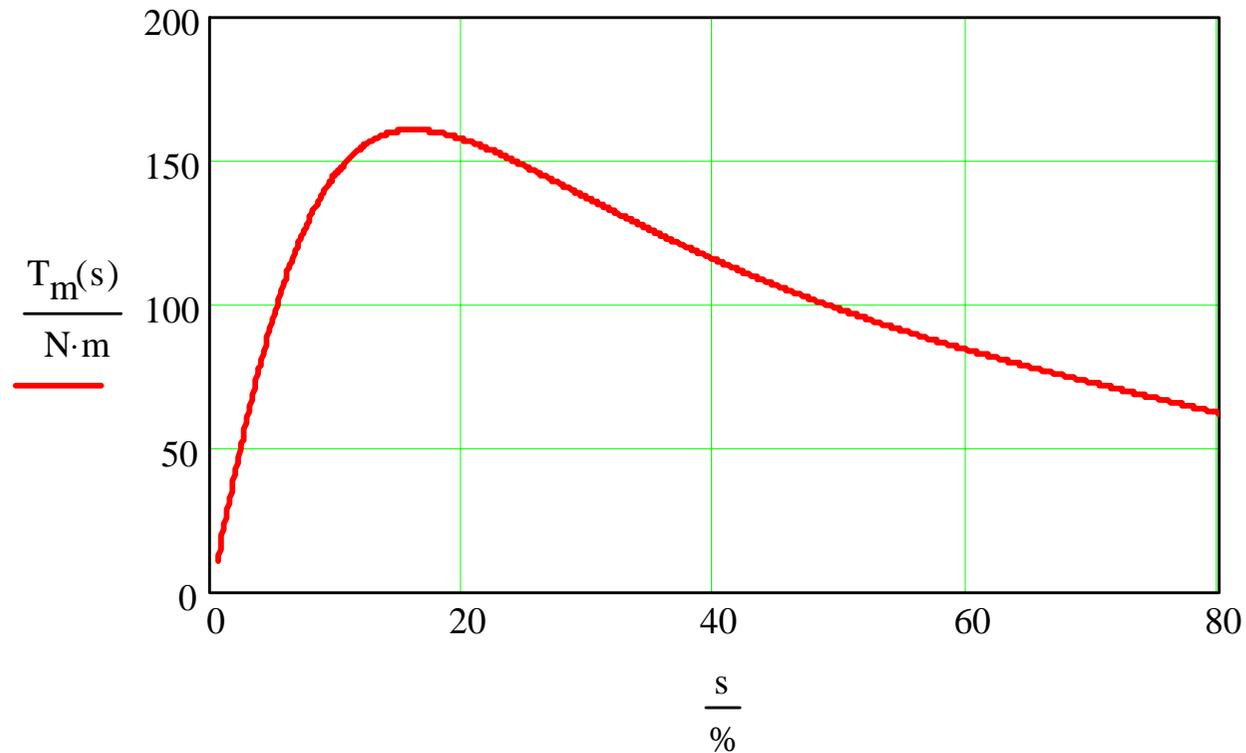
**Figure 25 Torque versus slip.**
