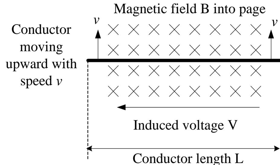
**Figure 14 Voltage induced in a conductor moving through a magnetic field.**
