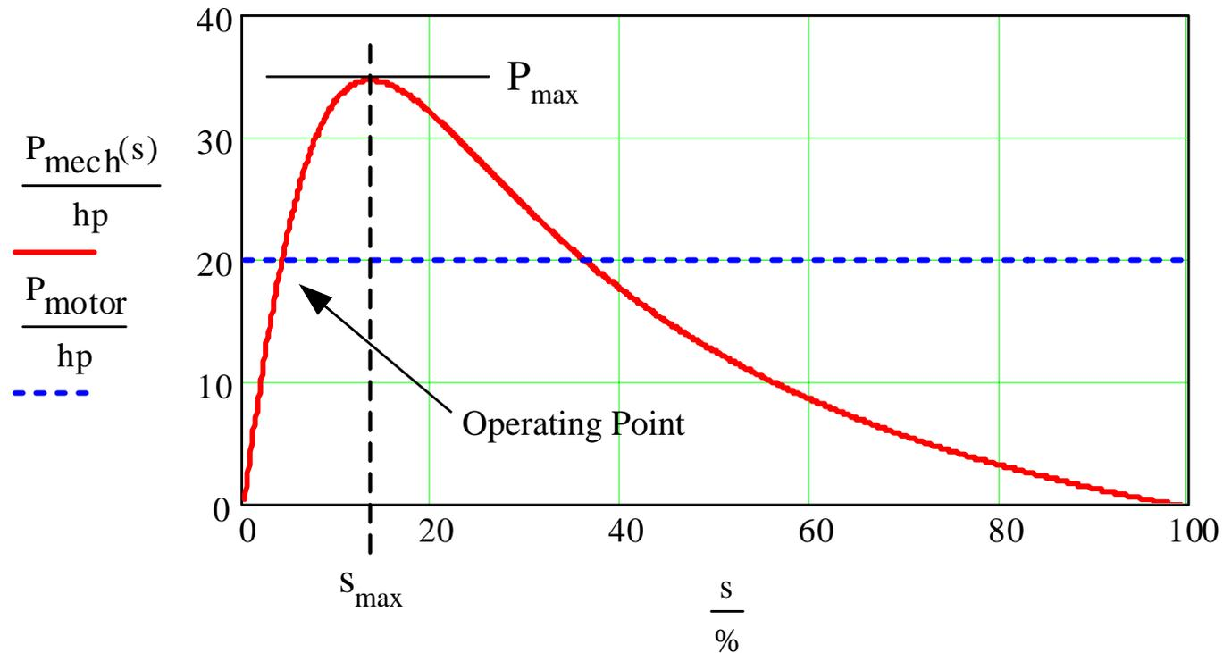
**Figure 24 Mechanical output power versus slip.**
