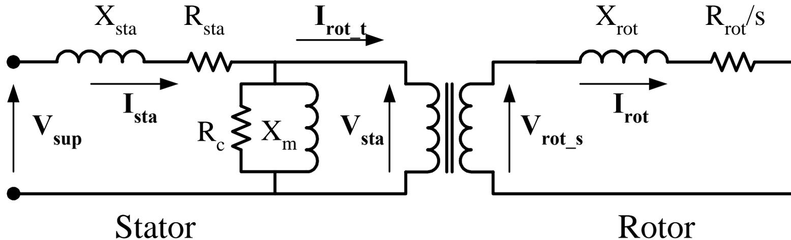
Figure 18 Modified equivalent circuit of a three-phase induction motor.
