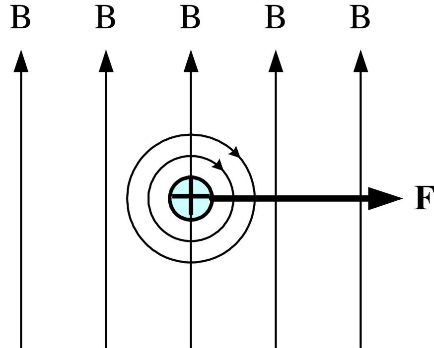
Figure 15 Force direction on a current-carrying conductor placed in a magnetic field ( $B$ ) (current into the page).
