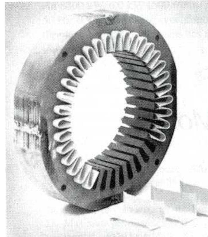
**Figure 5 Stator iron core without windings**
