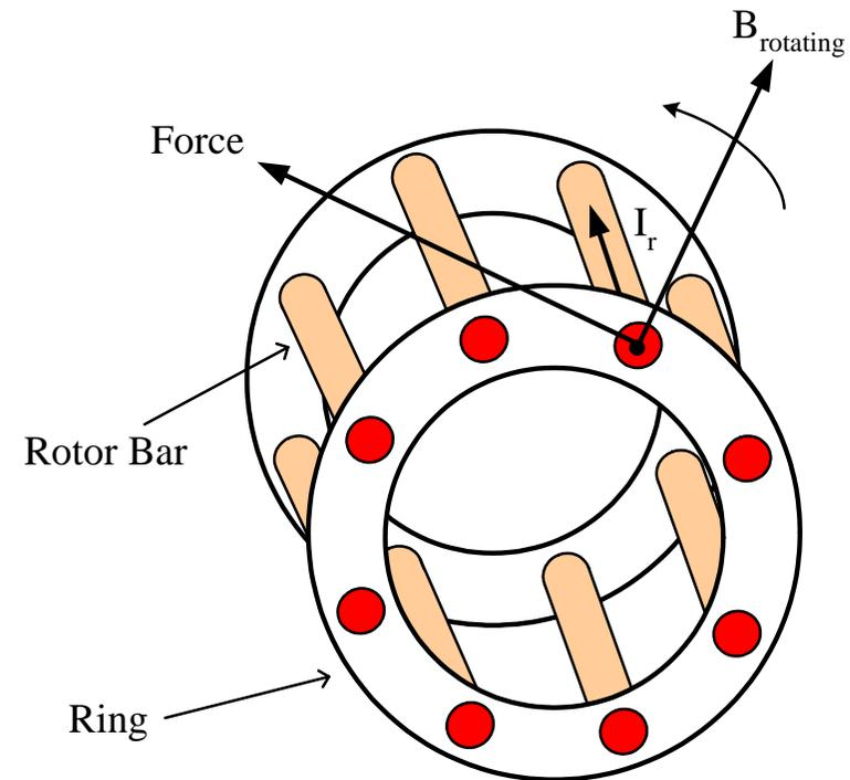
**Figure 16 Rotating magnetic field generated driving force.**
