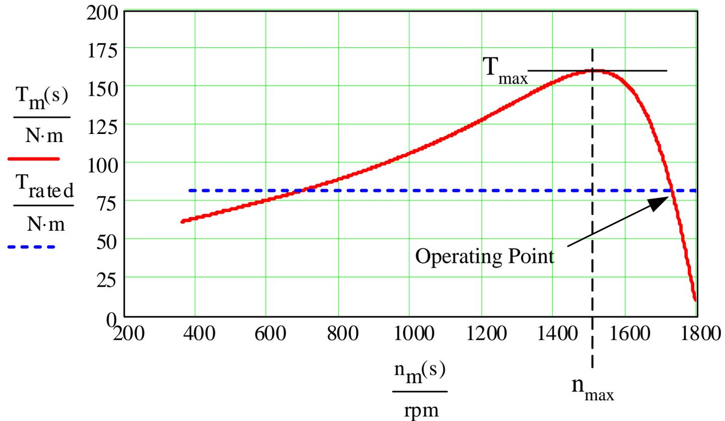
**Figure 26 Torque versus speed.**
