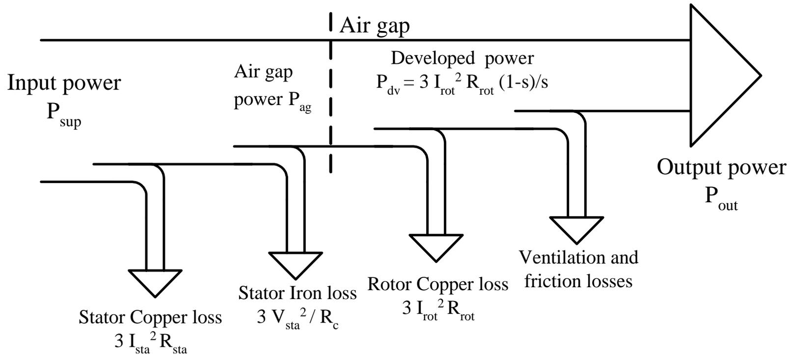
**Figure 21 Motor energy balance flow diagram.**
